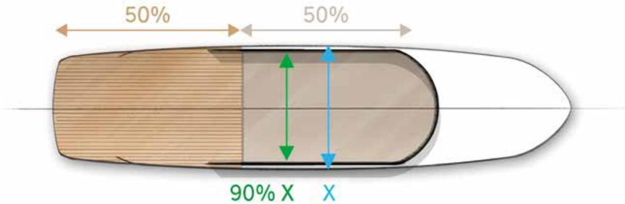
Redistribution and blending together of interior and exterior living spaces by greatly increasing the cockpit size.
