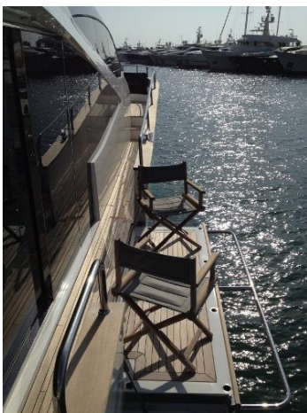
Dropdown bulwark balcony
